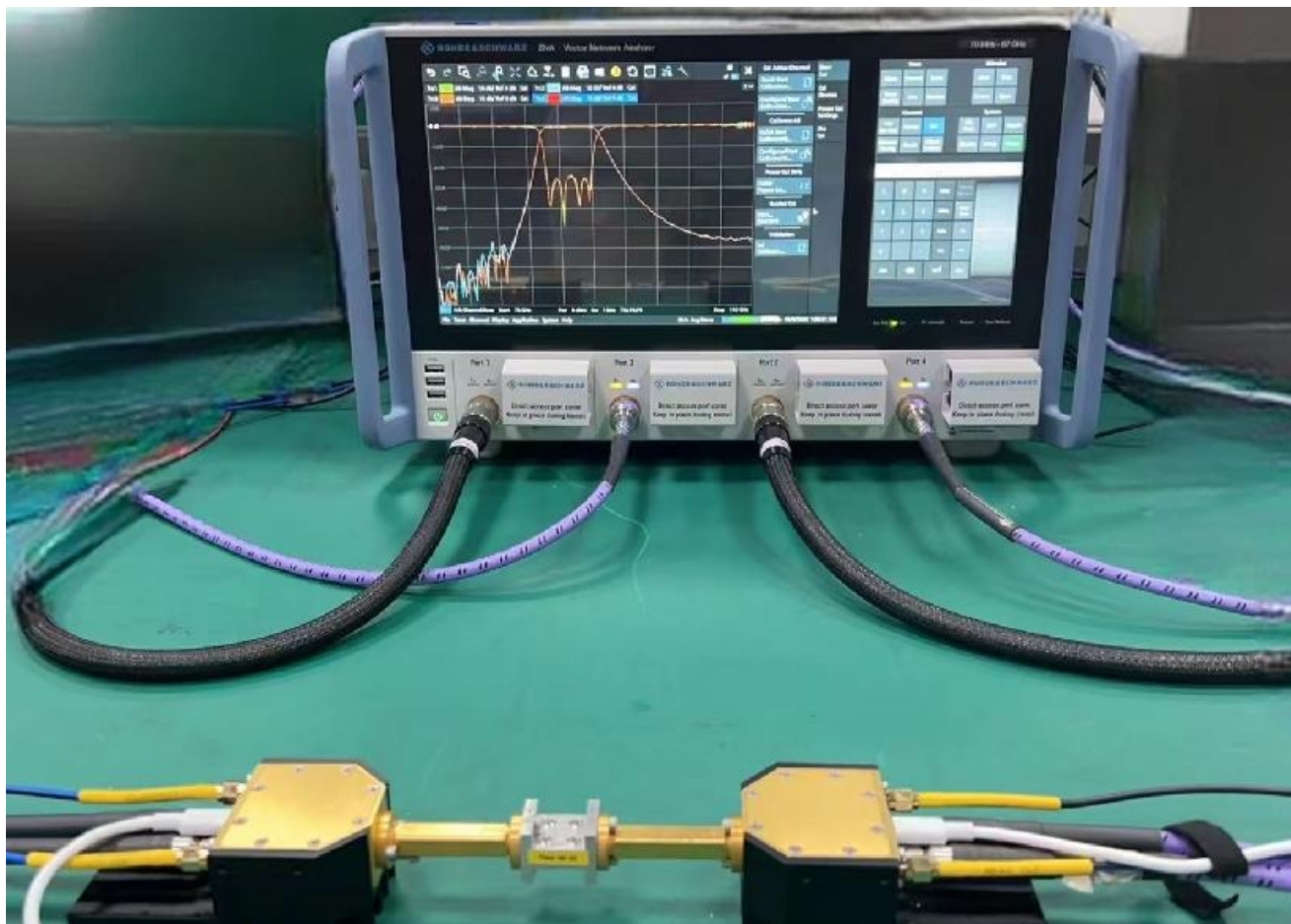
QS-1000TRs connection test with R&S VNA
